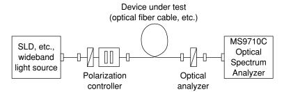
Convert the light from a wideband light source to a polarized wave using a polarization controller; pass this polarized light through the device under test, and input it to the MS9710C through an analyzer. The MS9710C measures the optical power polarization wavelength changes and calculates the PMD.
