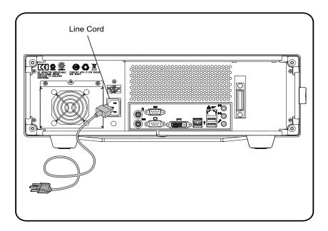
The product can operate from any single-phase AC power source supplying 100-240~V in the frequency range from 50-60~Hz. The maximum power consumption is 240 W. The power supply automatically adapts to the applied AC power (Auto Selection) and monitors the AC power range. The mains supply voltage fluctuation shall not exceed 10% of the specified supply voltage.
