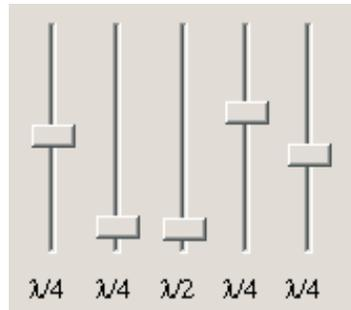
You can store five sets of slider positions by pressing **CTRL** while clicking on a memory button of the control bar. All five waveplate positions are stored for each memory button. Simply click on the desired memory button to recall this set any time later.
