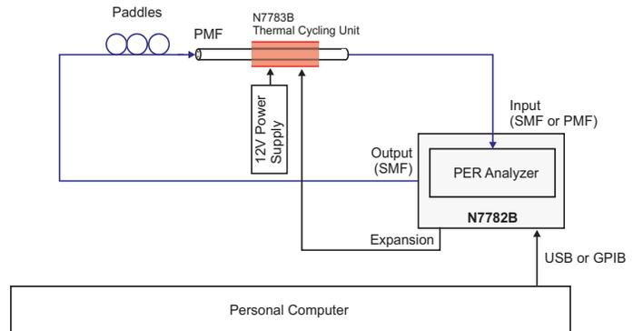
Figure 3 N7782B with internal laser source and N7783B Setup
