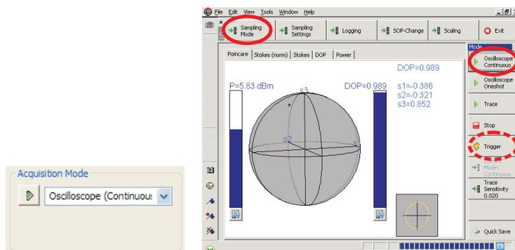
There are two options in this mode: Continuous and Oneshot. In the continuous mode, the measurement is restarted after receiving a trace. In oneshot mode the acquisition has to be manually (re)started by pressing the button next to the list box or by pressing **Trigger**, when using the Integrated PC Mode. To stop measuring in continuous mode select **Hold** from the drop-down menu or by pressing **Stop** respectively.
