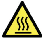
This label is located near certain parts of the instrument that get hot during operation. This applies to the white surface below the lid of the N7783B Thermal Cycling Unit, i.e. the trench that the fiber is placed into. Avoid touching this surface during operation.
