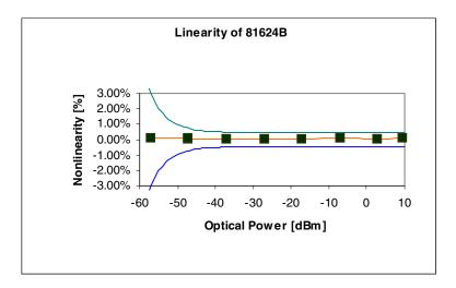
Figure 12 Example of Linearity Test Result.
