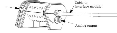
Figure 1 Rear view of an Optical Head with Analog Output
