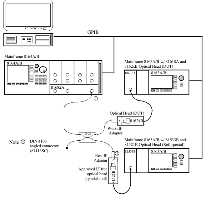
Figure 16 Setup for Relative Uncertainty due to Interference Measurement
