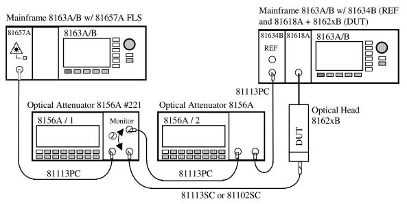
Figure 11 Measurement Setup for Power Linearity
