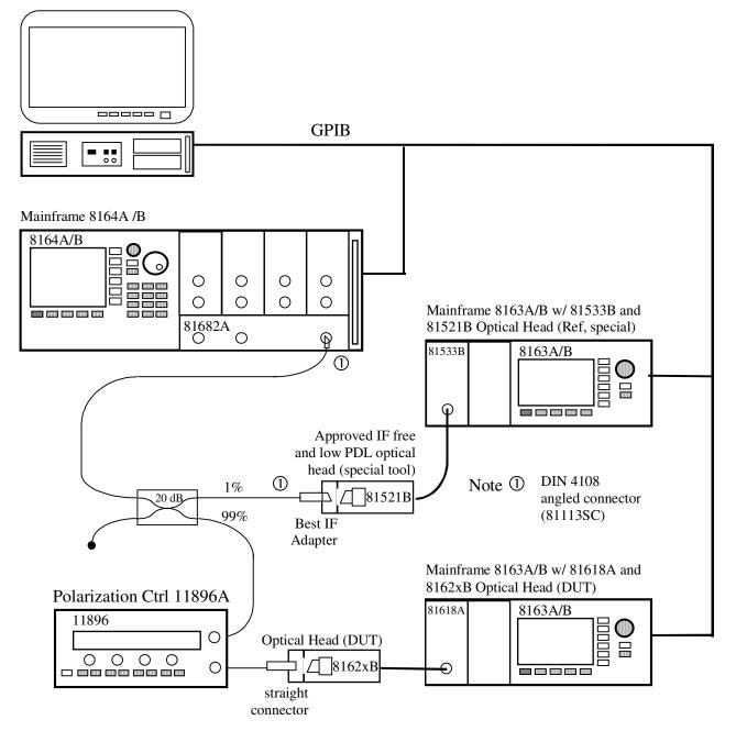
Figure 15 Measurement Setup for PDL Test
