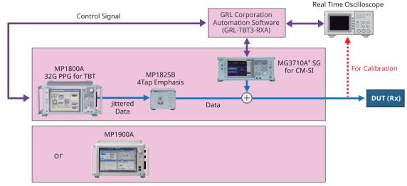
★: The MG3710A is used at common mode noise loads.
