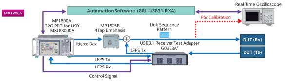
★: G0373A is used for LFPS (Low Frequency Periodic Signal) generation and BER measurement.
