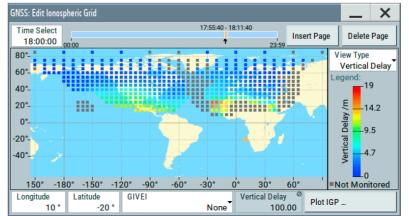
Configuration and simulation of ionospheric path delays with the R&S\*SMBV100B
