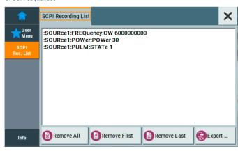
The R&S°SMBV100B helps users quickly and correctly create remote control programs. The instrument's built-in SCPI macro recorder with code generator can automatically record all manual settings and create an executable MATLAB° script. The R&S°SMBV100B therefore helps minimize the time required for test automation, saving development resources.
