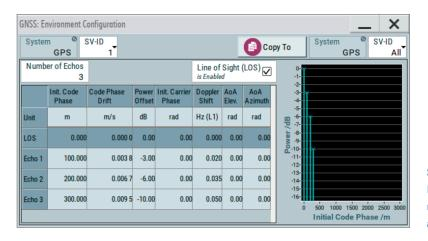
Simulation of multipath propagation for SV 1 with the R&S\*SMBV100B. In addition to the line of sight, three reflections with different relative delays, relative amplitudes and relative Doppler shifts are present
